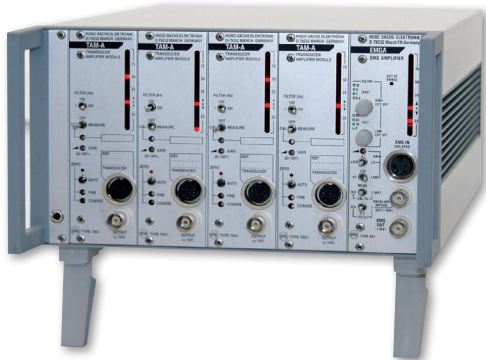
PLUGSYS Housing Type 601 with Five PLUGSYS Modules
